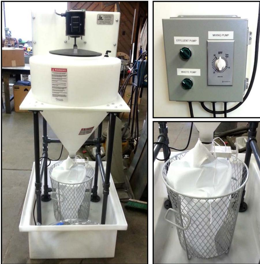
A&B Deburring's effluent recycling system offers a simple and cost-effective approach in the separation and disposal of waste created from vibratory finishing operations.
